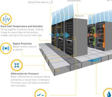
Contact Closure The dual contact closure is used with 3rd party sensors such as smoke detectors magnetic door locks, or to trigger webcams whenever a cabinet door is opened.
